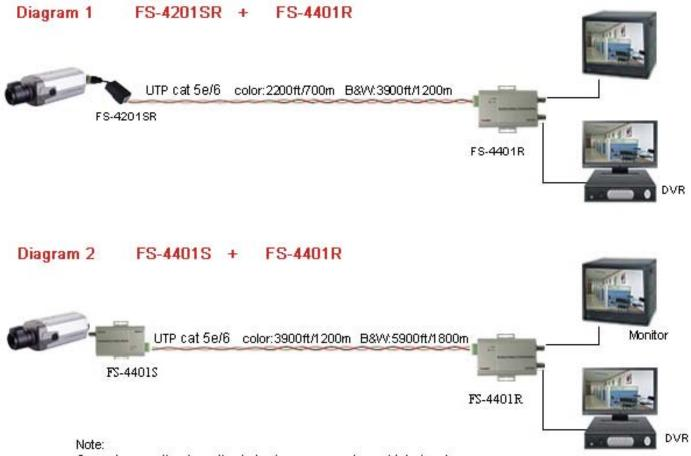
Ground connection for active balun is necessary to avoid device damage
