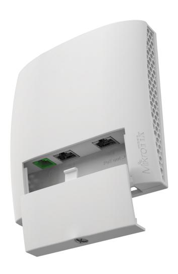
The wsAP has three Ethernet ports: one on the back side for easy PoE-in, and two LAN ports behind the front door. The device provides Dual concurrent 2.4 GHz and 5 GHz WiFi coverage, it supports 802.11ac, as well as legacy standards. A USB 2.0 port is provided, to charge mobile devices or for storage.
